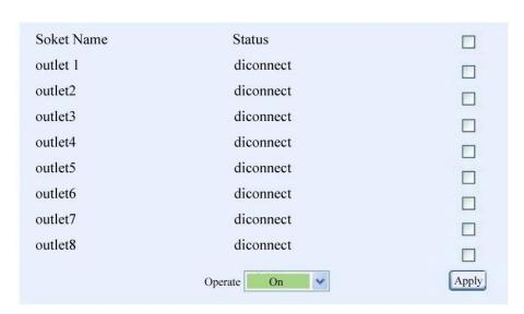
In this interface, the 8-way output of LIU-0832-WN can be set to be turned on and off.
