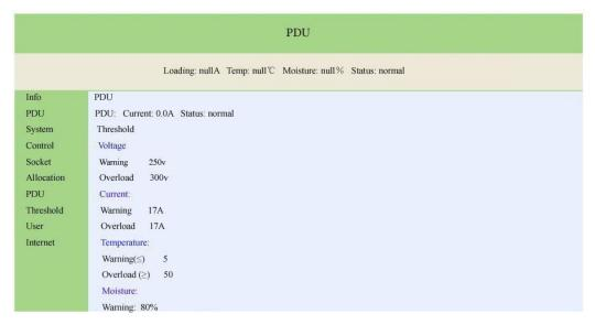
2.System information of the PDU Click "System" in the information bar on the left side of the interface to display the system information of the PDU, as shown below.
