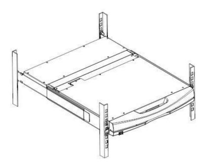
4. Use the screws supplied with this package to attach the bars to the rear of the switch. At this point, you have completed the rack mounting of the LCD KVM switch for subsequent use.
