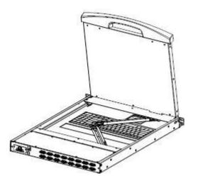
2. Remove the KVM assembly and the front LCD assembly by removing the KVM assembly and the mounting screws on the brackets on both sides as shown.
