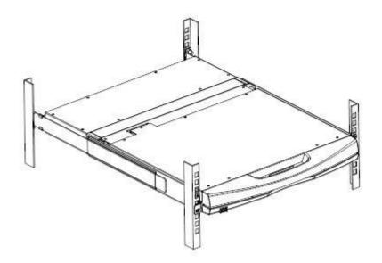
3. Slide the rear attachment slide bracket along the side strips until it reaches the rear of the switch.
