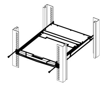
4. Use the screws supplied with this package to attach the bars to the rear of the switch. At this point, you have completed the rack mounting of the LCD KVM switch for subsequent use.
