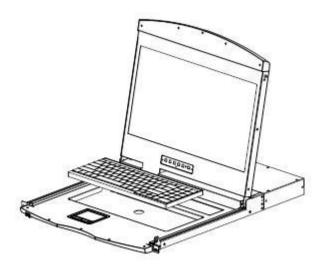
3. Pull the keyboard out of the limit slot, find the USB port on the connection, and remove the USB Type A connector from the interface.
