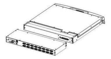
3.Disassembly and installation process Pay attention to the interface between the KVM module and the LCD module.Otherwise,the connection interface may be damaged and the device function may be caused. Invalid.
