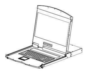
2. There is a circular hole at the bottom of the keyboard panel. You can use your finger to pass the circular hole to lift the keyboard up.
