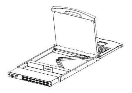
3. Replace the KVM module at the rear of the LCD. Fix the screws in the corresponding screw holes as shown in the figure, and then fix the whole machine in the cabinet according to the corresponding steps.
