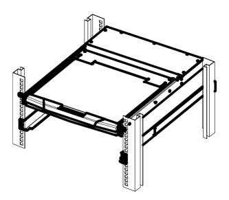
2. Slide the switch onto the support flanges. Use the screws supplied with this package **t**o loosely attach the front of the switch to the front of the rack.
