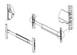
2.Slide the LCD KVM device into the support flange, use screw in this package provided with wire front portion of this switch is fixed to the front of the rack and locked.
