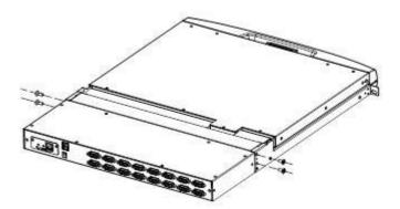
For single-port HDMI KVM connection, please connect the interface adapter module as shown below.
