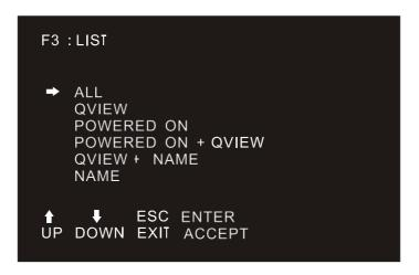
Many of the OSD functions only operate on the computers that have been selected for listing on the main screen with this function. The choices and their meanings are given in the table below:
