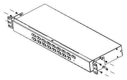
3. Install the KVM switch with the mounting plate attached to the rack, and align the mounting hole of the mounting plate with the mounting hole on the rack. Use the rack mounting screws in the mounting bracket to secure the mounting plate to the front end of the racktight.
