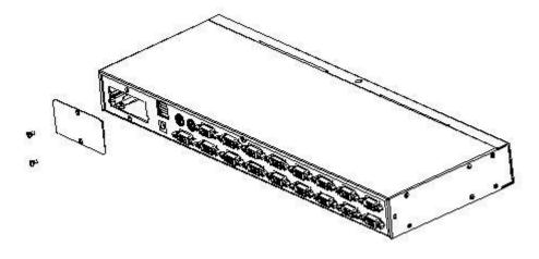
2. Take the extended IP module and push it gently into the recess in the mounting module cavity as shown.
