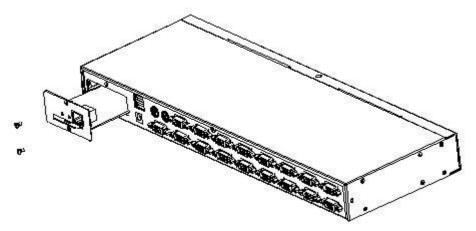
4. After finishing the installation of the IP module, please follow the instructions of the IP module user manual to install the software and network IP configuration of the device before connecting the network cable to the switching equipment. Then, you can access the network to log in to use. (For details, refer to the IP module's user manual.)
