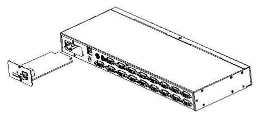
3. Push the IP module to the bottom, and then tighten the IP module with the two screws which removed from the front panel.
